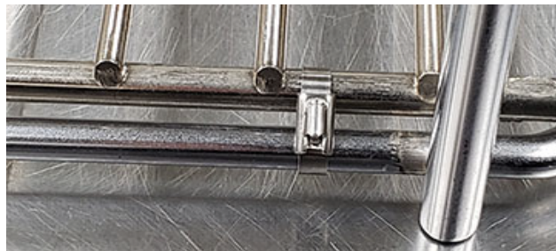
Close-up of zip tie in place (older style rack)
